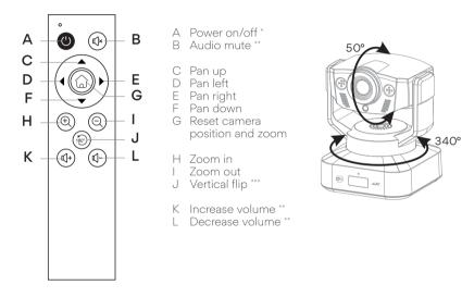
\* The **Power on/off** button on the remote and on the camera body work independently. If the camera is powered off via the **Power button** on the camera body, the red **Power indicator** light will light up to indicate that the master power switch has been used and the remote is disabled
