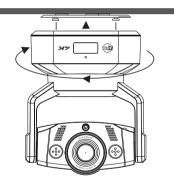
Push the camera against the mounting plate and rotate it clockwise.
