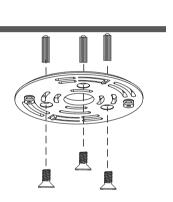
Use the included hardware to attach the mounting plate to the ceiling as shown. Point the arrow on the mounting plate in the direction you want the camera to face.
